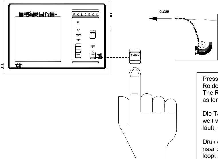
Press button "close" and bring the Roldeck to the correct closed position. The Roldeck motor will continue to run as long as the button remains pressed in.
