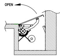
Press button "open" and bring the Roldeck to the correct open position.
