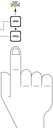
Press buttons " prog" and "open" simultaneously to record this position in the memory. ( yellow LED "open" burns)
