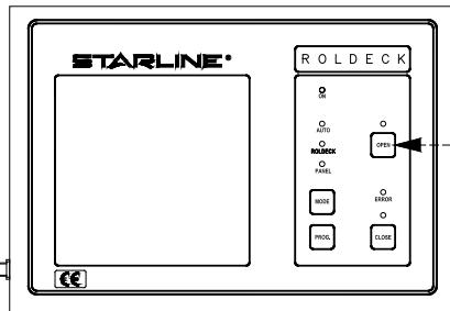
Press button "open" and bring the Roldeck to the correct open position.
