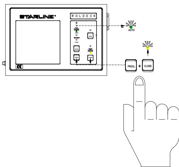
Press buttons "prog" and "close" simultaneously to record this position in the memory. (yellow LED "close" burns).
