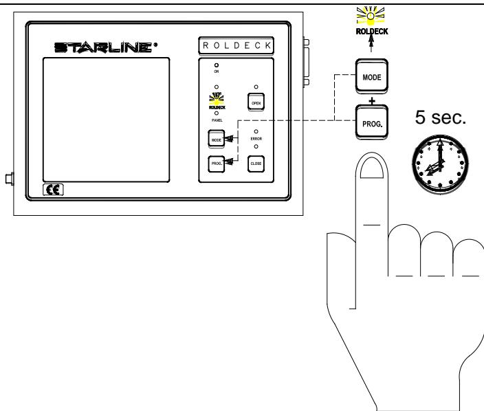
Press buttons "prog" + "mode"(ca. 5 sec.) simultaneously until the yellow Roldeck LED starts to flash. The Roldeck control has now been reset.
