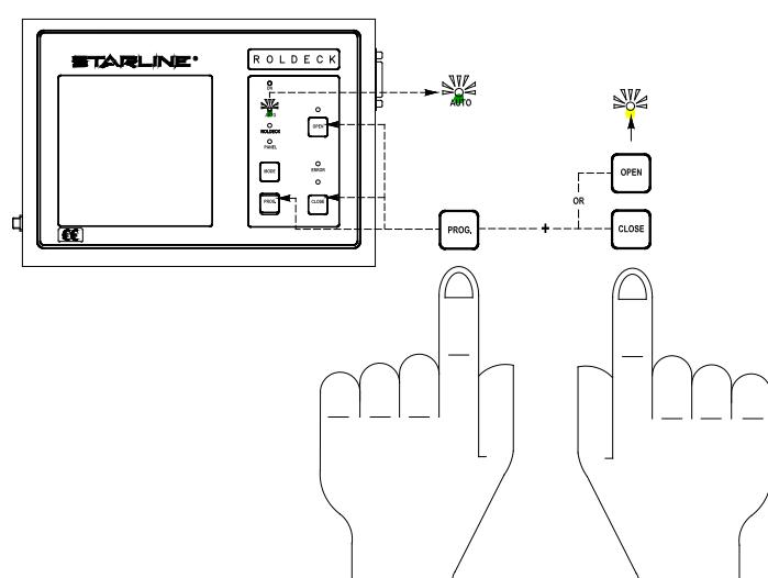
Confirm this position by pressing buttons „**prog**“ and either „**open**“ or „**close**“ simultaneously.
