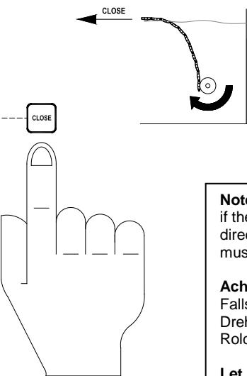
Press button "close" and bring the Roldeck to the correct closed position. The Roldeck motor will continue to run as long as the button remains pressed in.
