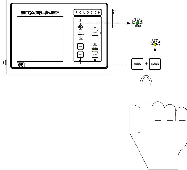
Press buttons “**prog**” and “**close**” simultaneously to record this position in the memory. (yellow LED “**close**” burns).
