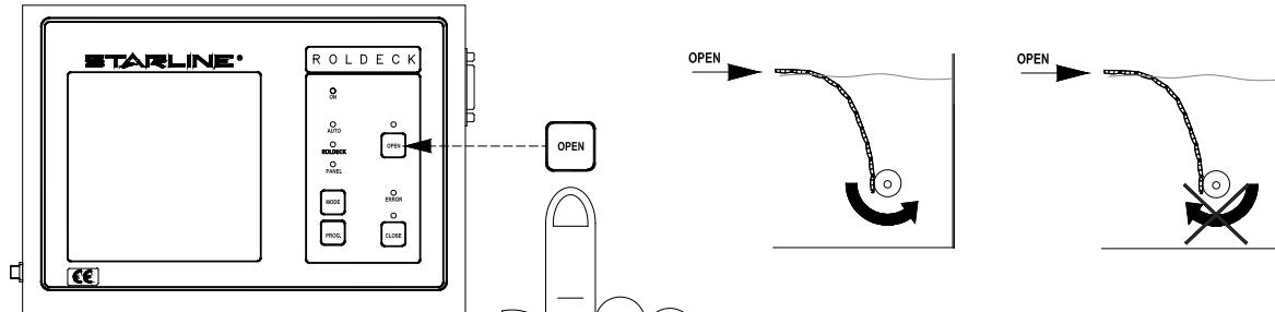
Press button "open" and bring the Roldeck to the correct open position.
