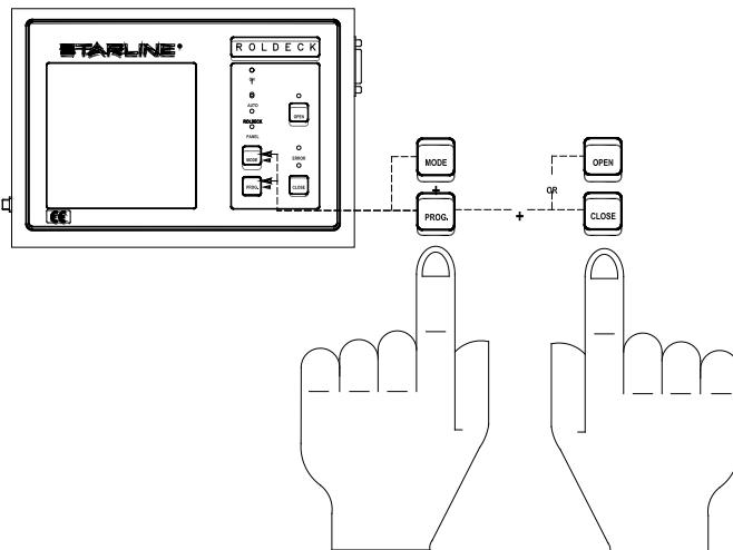
By pressing the "**mode**" button the Roldeck or the bottom flap can be selected for fine-tuning. The LED in "Rolleck" or "Panel" starts to burn.
